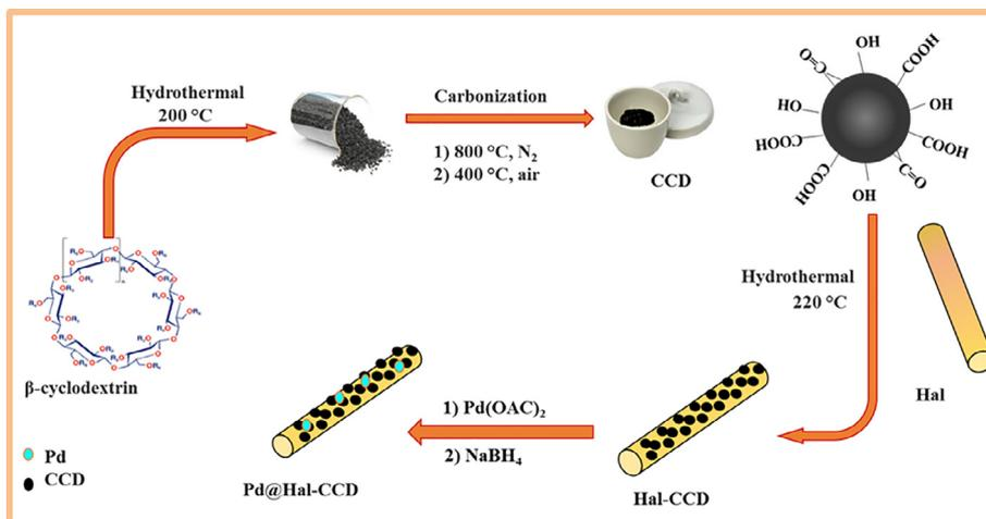
Fig. 1. The schematic protocol for the synthesis of Pd@Hal-CCD.
