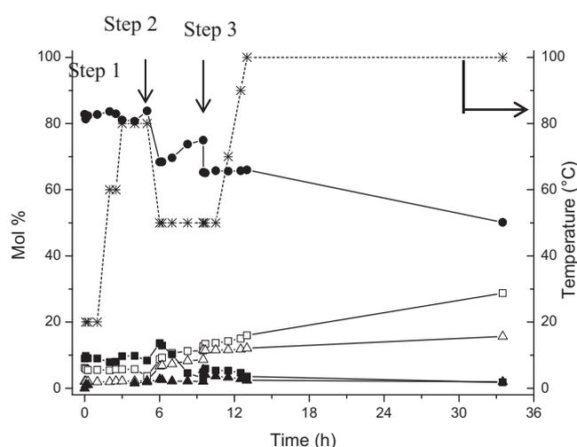
**Fig. 9.** Transformation of tetrahydropyran over Al<sub>2</sub>O<sub>3</sub> (step 1), MgO (step 2) and Cs-MCM-41 mesoporous catalyst (step 3). Symbols: tetrahydropyran (●), dioxinol (■), dehydration product 1 (□), unknown 1 (open triangle), unknown 2 (solid triangle) and temperature (\*).
