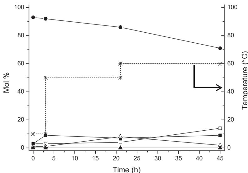
**Fig. 7.** Transformation of tetrahydropyran over Amberlite 120H. Symbols: tetrahydropyran (●), dioxinol (■), dehydration product 1 (□), unknown 1 (open triangle), unknown 2 (solid triangle) and temperature (\*).
