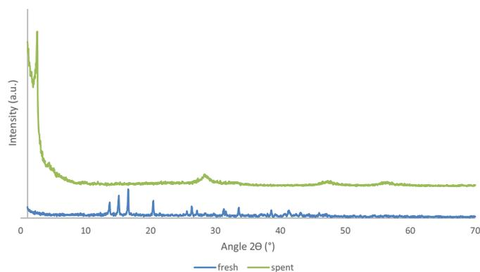
**Fig. 3.** X-ray powder diffraction patterns of fresh and spent mesoporous Ce composite.
