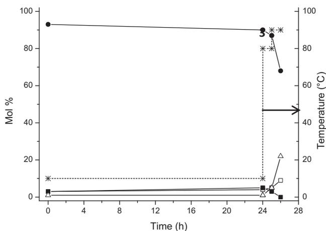
**Fig. 6.** Transformation of tetrahydropyran over H-Beta-25 zeolite catalyst. Symbols: tetrahydropyran (●), dioxinol (■), dehydration product 1 (open square), unknown products (open triangle) and temperature (\*).
