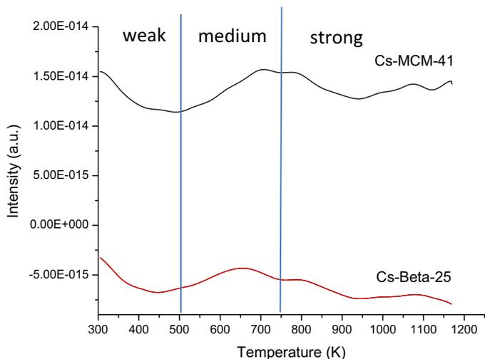
**Fig. 2.** TPD of CO<sub>2</sub> from Cs-MCM-41 mesoporous catalyst and Cs-Beta-25 zeolite catalyst determined by mass spectrometry.
