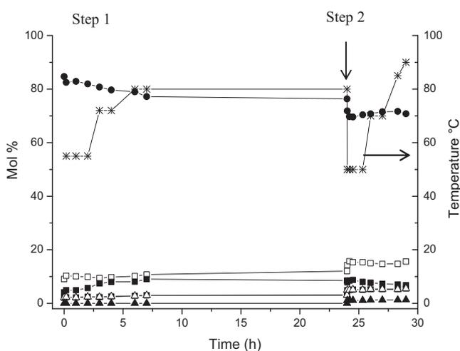
**Fig. 8.** Transformation of tetrahydropyran over Cs-Beta-25 (step 1) and Fe-Beta-300 (step 2). Symbols: tetrahydropyran (●), dioxinol (■), dehydration product 1 (□), unknown 1 (open triangle), unknown 2 (solid triangle) and temperature (\*).
