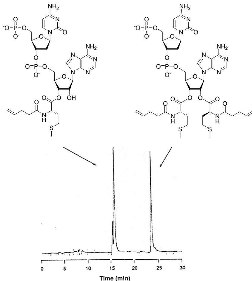
**Figure 2.** Separation of monomethionyl-pdCpAs from bismethionyl-pdCpA on  $C_{18}$  reversed phase HPLC. Monomethionyl-pdCpA eluted first as a mixture of (equilibrating) 2'- and 3'-*O*-aminoacyl derivatives (~16.0 and 16.5 min), followed by the bisacylated derivative (~24 min).
