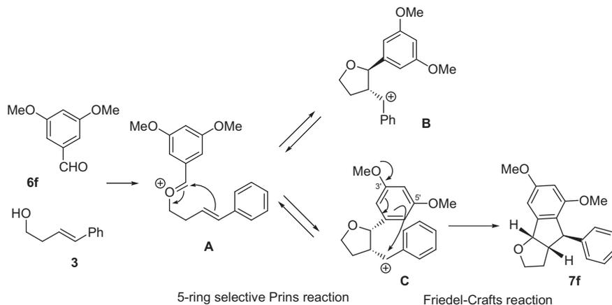
**Scheme 2.** Mechanism for the formation of **7**.
