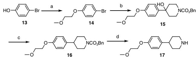
**Scheme 4.** Reagents and conditions: (a)  $K_2CO_3$ , 2-bromoethyl methyl ether,  $CH_3CN$ ,  $\Delta$ , 95%; (b) 1-*n*-BuLi,  $-78^\circ C$ , THF; 2-(4-oxopiperidin-1-yl)carboxylic acid benzyl ester,  $-78^\circ C$  to rt, 60%; (c)  $Et_3SiH$ , TFA,  $CH_2Cl_2$ ,  $-78^\circ C$  to rt, 95%; (d)  $H_2$ , 5% Pd/C, MeOH/EtOAc, 1 atm, 98%.
