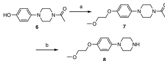
**Scheme 2.** Reagents and conditions: (a) 2-bromoethyl methyl ether, NaH, DMF, 60 °C, 80%; (b) 1–6 N HCl, 80 °C; 2–5 N NaOH, 95%.
