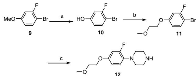
**Scheme 3.** Reagents and conditions: (a)  $\text{BBr}_3/\text{CH}_2\text{Cl}_2$ ,  $\Delta$ , 99%; (b)  $\text{K}_2\text{CO}_3$ , 2-bromoethyl methyl ether,  $\text{CH}_3\text{CN}$ ,  $\Delta$ , 98%; (c) piperazine,  $\text{Pd}_2(\text{dba})_3$ , NaO<sup>t</sup>Bu, BINAP, toluene,  $\Delta$ , 70%.
