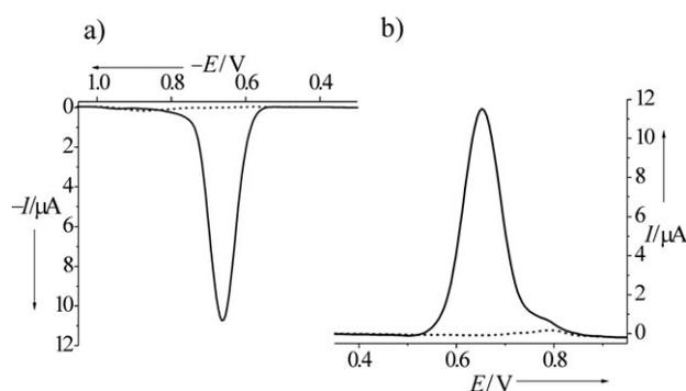
**Figure 2.** Square-wave voltammetry (SWV) signals resulting from a) nitro group reduction in dU<sup>NO<sub>2</sub></sup>-TP or b) amino group oxidation in dU<sup>NH<sub>2</sub></sup>-TP at a pyrolytic graphite electrode. Dotted curves correspond to unmodified dTTP. For more details, see the Supporting Information.
