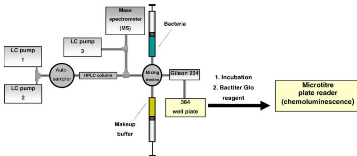
**Figure 1.** Schematic overview of the fully integrated MS-based high-resolution screening system. For details, refer to the text.
