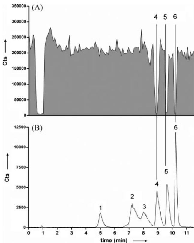
**Figure 4.** Separation with MS detection and simultaneous bioactivity screening of a 1:20 diluted neomycin shotgun reaction mixture: (A) the bioactivity trace and (B) the extracted-ion chromatogram for the ions with  $m/z$  727.5 + 364.3.
