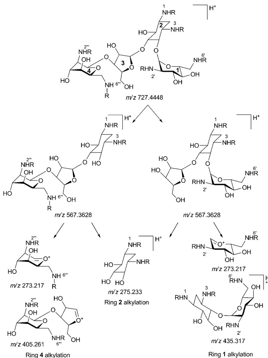
**Figure 7.** Fragmentation scheme of mono-*N*-alkyl neomycin derivatives in MS<sup>*n*</sup> experiments, showing the different ring losses and the calculated  $m/z$  values of the resulting fragment ions. R = *n*-octyl or H.
