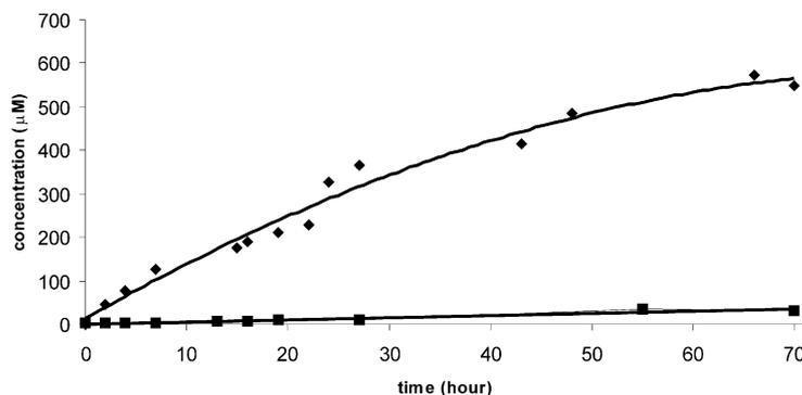
**Figure 5.** Determination of CPT release from the HPMA-copolymer by PGA versus background reaction in absence of PGA. -◆-?Complex **12** (330  $\mu\text{M}$ ) with PGA (4.4  $\mu\text{M}$  in PBS-7.4). -■- Complex **12** (330  $\mu\text{M}$ ) in PBS (pH 7.4). Reactions were incubated at 37 °C for the indicated time. The drug release concentration was monitored by HPLC analysis.
