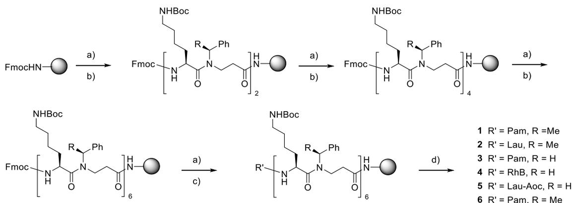
**Scheme 2** Assembly of  $\alpha$ -peptide/ $\beta$ -peptoid hybrids; shown with the use of tetrameric building blocks. Reagents and conditions: **a** 20% piperidine-DMF; **b** **10/11**, PyBOP/DIPEA, HBTU/DIPEA, or DIC/Oxyma, DMF; **c** End-group modification: Lau-OSu/Pam-OSu, DIPEA,  $\text{CH}_2\text{Cl}_2$ ; Fmoc-(S)-Aoc-OH or RhB, PyBOP, DIPEA, and
