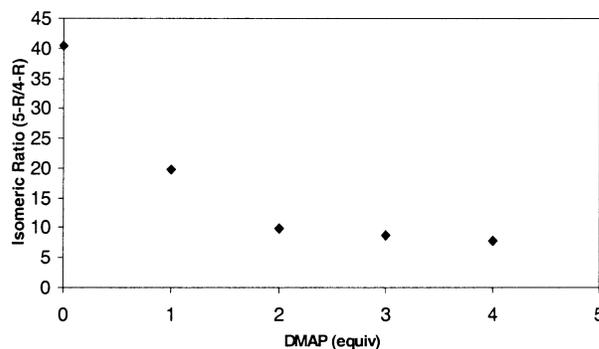
**Figure 2.** Ratio of 5-substituted to 4-substituted isomers in the reaction of CO<sub>2</sub> and *N*-propyl 2-phenylaziridine as a function of DMAP concentration. Reaction conditions: catalyst (12.6 mg, 0.02 mmol, 1 equiv), *N*-propyl-2-phenylaziridine (0.322 g, 2 mmol, 100 equiv), 400 psig of CO<sub>2</sub>, CH<sub>2</sub>Cl<sub>2</sub> (3.7 mL), 100 °C, 120 min.
