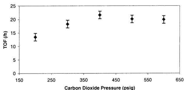
**Figure 4.** Activity of the (salen)chromium(III)/DMAP catalyst system as a function of CO<sub>2</sub> pressure in the reaction of CO<sub>2</sub> and *N*-propyl-2-phenylaziridine. Reaction conditions: catalyst (12.6 mg, 0.02 mmol, 1 equiv), DMAP (2 equiv), *N*-propyl-2-phenylaziridine (0.322 g, 2 mmol, 100 equiv), CH<sub>2</sub>Cl<sub>2</sub> (3.7 mL), 400 psig of CO<sub>2</sub>, 100 °C, 60 min.
