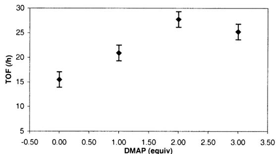
**Figure 1.** Activity of (salen)chromium(III)/DMAP as a function of DMAP concentration in the reaction of CO<sub>2</sub> and *N*-propyl-2-phenylaziridine. Reaction conditions: catalyst (12.6 mg, 0.02 mmol, 1 equiv), 400 psig of CO<sub>2</sub>, *N*-propyl-2-phenylaziridine (0.322 g, 2 mmol, 100 equiv), CH<sub>2</sub>Cl<sub>2</sub> (3.7 mL), 100 °C, 120 min.
