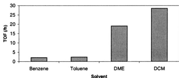
**Figure 3.** Activity of the (salen)chromium(III)/DMAP catalyst as a function of solvent in the reaction of CO<sub>2</sub> and *N*-propyl-2-phenylaziridine. Reaction conditions: catalyst (12.6 mg, 0.02 mmol, 1 equiv), DMAP (2 equiv), *N*-propyl-2-phenylaziridine (0.322 g, 2 mmol, 100 equiv), solvent (3.7 mL), 400 psig of CO<sub>2</sub>, 100 °C, 120 min.
