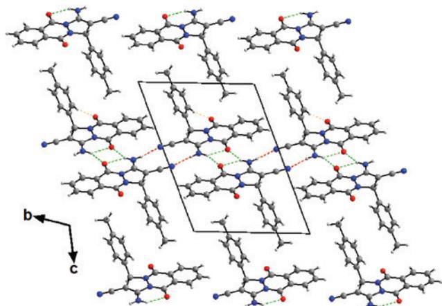
**Fig. 3:** N–H...O and N–H...N hydrogen bond interactions resulting in the formation of an infinite two-dimensional network of compound **4c** in the crystal (in red N–H...N and in green N–H...O).**Table 4:** Hydrogen bond distances (Å) and angles (deg) for **4c**.
