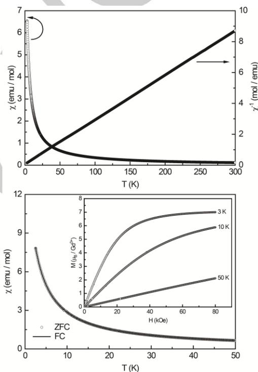
**Figure 5.** Magnetic properties of  $\text{Gd}_4(\text{OH})_2(\text{N}_3)_{10} \cdot 10 \text{ DMSO}$ : (top) temperature dependence of the magnetic susceptibility ( $\chi$  and  $\chi^{-1}$  data) measured at 10 kOe; (bottom) zero-field-cooled / field cooled (ZFC/FC) measurements at 100 Oe; (bottom inset) magnetization isotherms at 3, 10 and 50 K.
