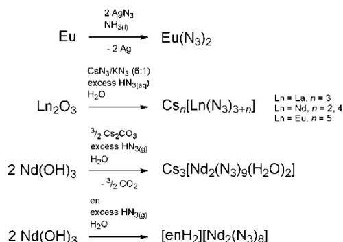
**Scheme 2.** Preparation of  $\text{Eu}(\text{N}_3)_2$ ,  $\text{Cs}_3[\text{La}(\text{N}_3)_6]$ ,  $\text{Cs}_2[\text{Nd}(\text{N}_3)_5]$ ,  $\text{Cs}_4[\text{Nd}(\text{N}_3)_7]$ ,  $\text{Cs}_5[\text{Eu}(\text{N}_3)_8]$ ,  $\text{Cs}_3[\text{Nd}_2(\text{N}_3)_9(\text{H}_2\text{O})_2]$  and  $[\text{enH}_2][\text{Nd}_2(\text{N}_3)_8]$  (en = ethylenediamine).
