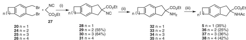
**Scheme 3** Synthesis of linearly annulated indane-based  $\alpha$ -amino acid derivatives. *Reagents and conditions:* (i) K<sub>2</sub>CO<sub>3</sub>, TBAHS, MeCN, reflux, 12–20 h; (ii) EtOH, dil. HCl, r.t., 12 h; (iii) Ac<sub>2</sub>O, DMAP, CH<sub>2</sub>Cl<sub>2</sub>, r.t., 12–24 h.
