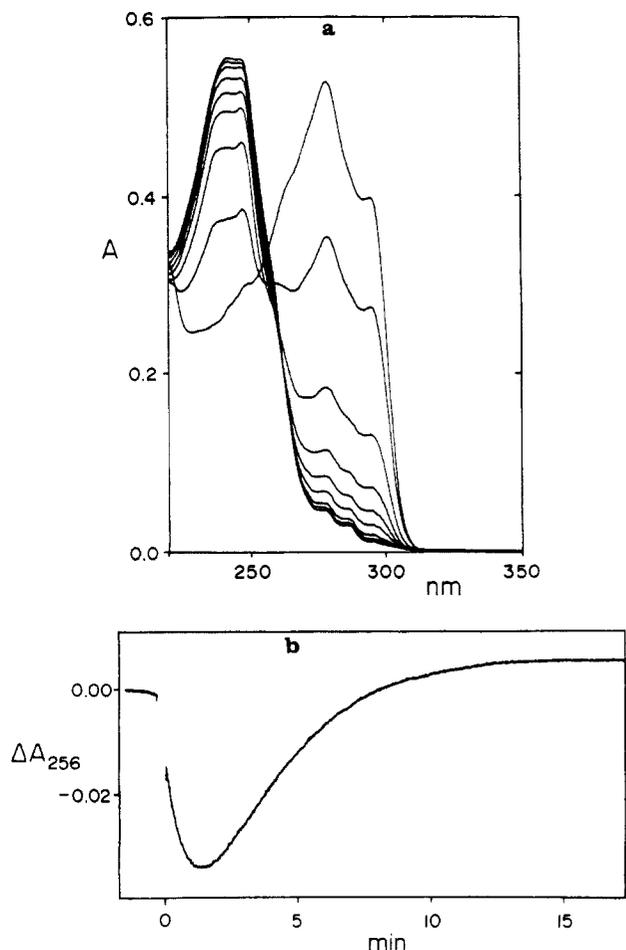
**Figure 3.** (a) Ultraviolet spectra of ynenol lactone **1f**, 25  $\mu\text{M}$  in 1.0 mL of  $\text{H}_2\text{O}$ . After the first spectrum ( $\lambda_{\text{max}}$  279 nm), 5  $\mu\text{L}$  of 10 mM NaOH was added, and spectra were recorded at 2-min intervals. (b) Time course of the same reaction, monitored at 256 nm. NaOH (30  $\mu\text{L}$  of 10 mM) was added at time zero.
