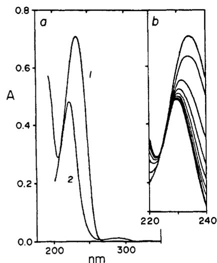
**Figure 1.** (a) Spectrum 1 is of 50  $\mu\text{M}$  **1a** in 1.0 mL of water, 25  $^\circ\text{C}$ . The pH was raised by addition of 10  $\mu\text{L}$  of 50 mM borate buffer, pH 10, and spectrum 2 was taken approximately 10 min later. (b) Time course of the same reaction recorded at 1-min intervals after the pH change.
