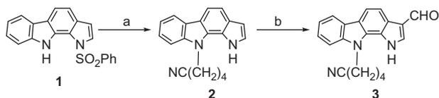
**Scheme 1.** Synthesis of nitrile derivative **3**. Reagents and conditions: (a) (i) 5-bromopentanenitrile, *t*BuOK, DMF, (ii) NaOH, MeOH, 86%; (b) POCl<sub>3</sub>, DMF, MW, 64%.
