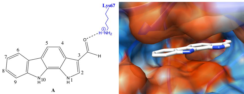
**Figure 1.** Binding of compound **A** to Pim-1 ATP binding site (surfaces are colored in orange-red (hydrophobic) and in blue (hydrophilic)) [**8**, PDB 3JPV]. H-bond indicated in dashed line.
