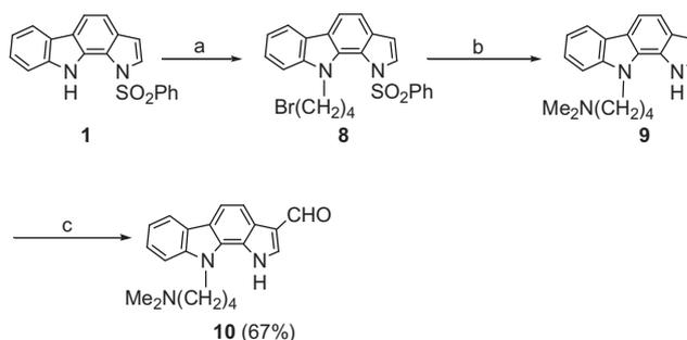
**Scheme 3.** Preparation of compound **10**. Reagents and conditions: (a) 1,4-dibromobutane, NaH, 84%; (b) (i) Me<sub>2</sub>NH–HCl, K<sub>2</sub>CO<sub>3</sub>, KI, THF, (ii) NaOH, MeOH, 57%; (c) (i) (COCl)<sub>2</sub>, DMF, CH<sub>2</sub>Cl<sub>2</sub>, (ii) NaOH, 67%.
