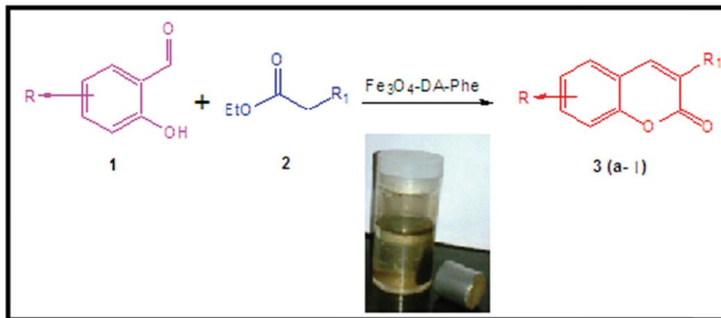
**Scheme 2.** Synthesis of coumarins by Knoevenagel condensation using Fe<sub>3</sub>O<sub>4</sub>-DA-Phe.
