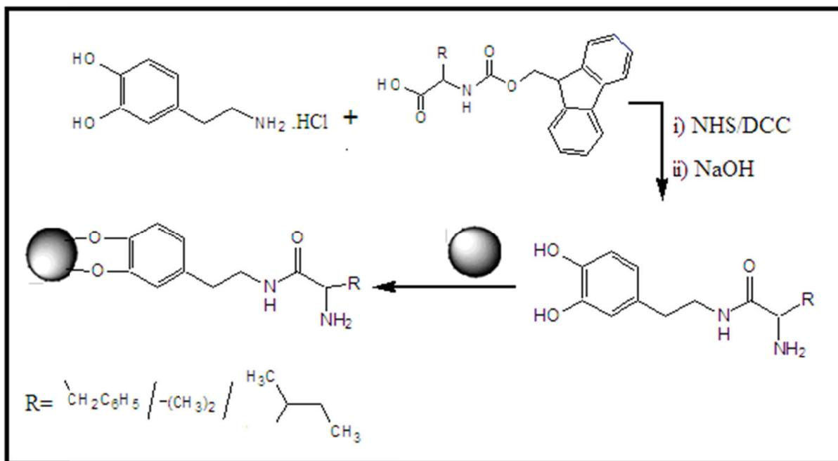
**Scheme 1.** Synthesis of functionalized iron oxide nanoparticle supported-amino acids ((Fe<sub>3</sub>O<sub>4</sub>-DA-Phe), (Fe<sub>3</sub>O<sub>4</sub>-DA-Val) and (Fe<sub>3</sub>O<sub>4</sub>-DA-Ile)).
