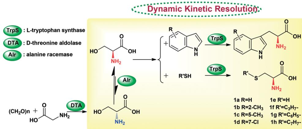
Scheme 1. Enzymatic synthesis of L-ncAAs from Gly and (CH<sub>2</sub>O)<sub>n</sub> using DTA, Alr and TrpS.
