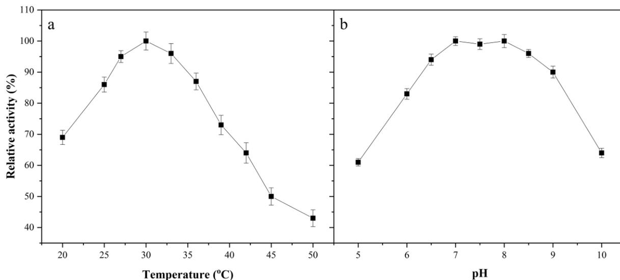
Figure 1. The effect of pH and temperature on DTA activity. The reaction (volume: 10 mL) was carried out at 200 rpm, in which DTA dry whole cell (5 mg), Gly (2.5 M), (CH<sub>2</sub>O)<sub>n</sub> (2.5 M) and PLP (0.4 mM) were contained. The mixture was shaken for 2 h at 30 °C for determination of the optimal pH and was shaken at pH 7 for determination of the optimal temperature. 100 % relative activity denoted that 16 % conversion of Gly or (CH<sub>2</sub>O)<sub>n</sub>.
