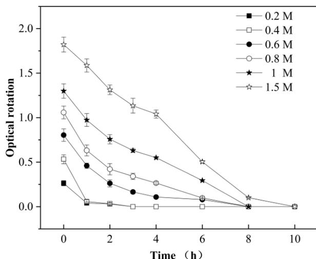
Figure 3. The effect of D-Ser concentration on Alr activity. The mixture (100 mL, pH 8.5) containing D-Ser, Alr dry whole cell (50 mg) and PLP (0.4 mM) reacted at 40 °C, 200 rpm.
