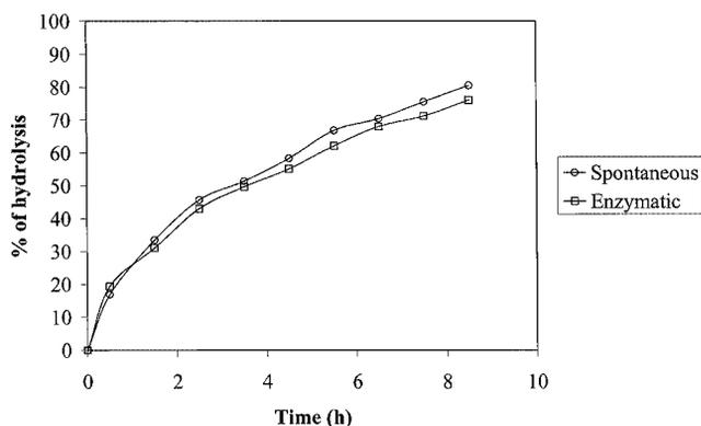
Figure 1. Comparison between spontaneous and enzymatically catalyzed hydrolysis of  $\alpha$ -glucosyl fluoride {experimental conditions: E338G glycosynthase,  $T = 55^\circ\text{C}$ ,  $\text{pH} = 7.8$ ,  $[\alpha\text{-GlcF}] = 50\text{ mmolL}^{-1}$ }.
