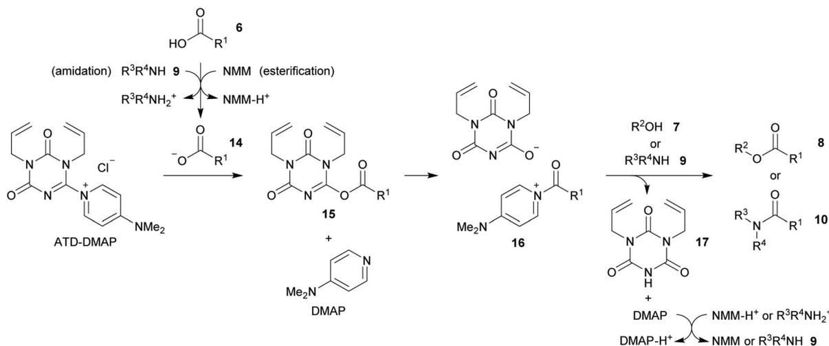
Fig. 4 Plausible reaction mechanism for esterification and amidation using ATD-DMAP.
