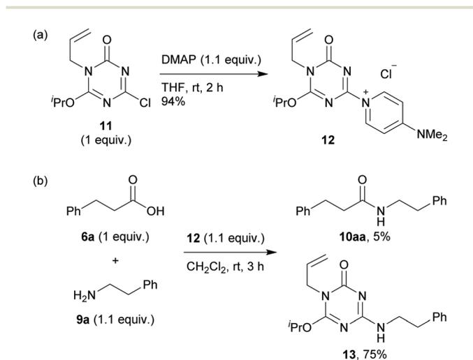
Fig. 3 (a) Preparation of triazinone-based reagent **12** containing DMAP and (b) attempted amidation using **12**.
