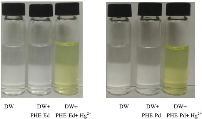
**Fig. 12** The color change of **PHE-Ed** and **PHE-Pd** in real samples of drinking water (DW)
