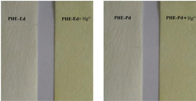
**Fig. 11** The filter paper test strips of **PHE-Ed** and **PHE-Pd** in DMSO, treated with  $\text{Hg}^{2+}$  solution ( $10^{-5}$  M) in water
