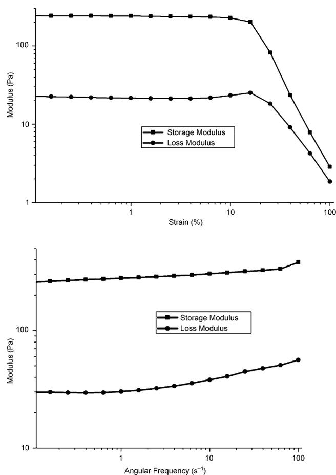
Figure 6. Rheological study of the hydrogel. Top: the amplitude-sweep study shows that the storage modulus ( $G' \approx 300$  Pa) was higher than the loss modulus ( $G'' \approx 37$  Pa), as expected for gels; bottom: the frequency-sweep study shows the characteristic features of a gel that was formed by an entangled network of fibers.
