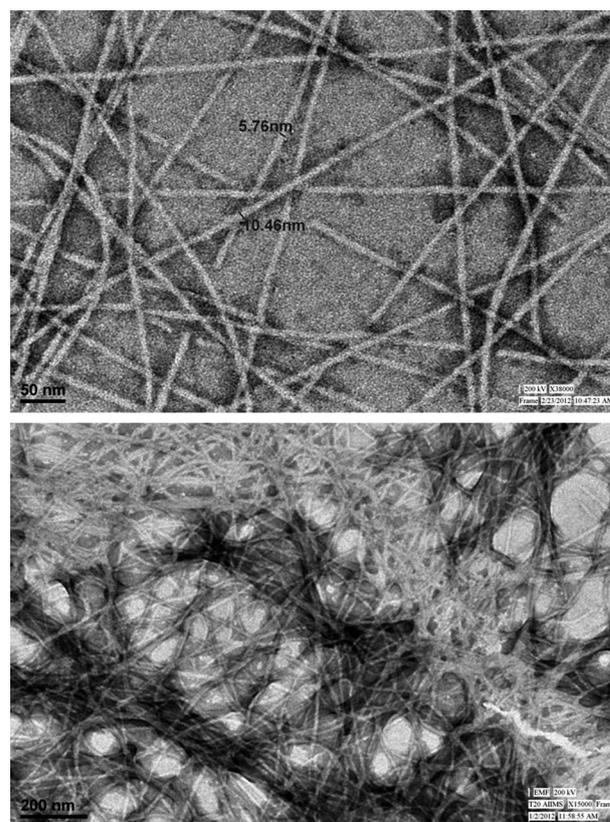
Figure 5. TEM images of gel fibers that were stained with phosphotungstic acid. Top: Thin, high aspect-ratio fibrillar assemblies with diameters of about 5 nm and lengths of a few microns; bottom: a dense mesh of the fibers that entrapped water molecules.
