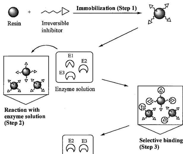
**Fig. 1.** Schematic Representation of Removal of Proteases by Covalent Chromatographic Technique Using Irreversible Protease Inhibitors.
