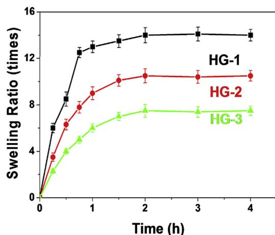
Fig. 2. Swelling ratios of the hydrogels with different content of C18 as a function of swelling time in deionized water.
