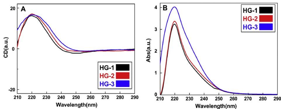
Fig. 5. CD (A) and UV-vis (B) spectra of the hydrogels with varied contents of C18, measured by placing the swollen hydrogels between two pieces of quartz glass at room temperature.
