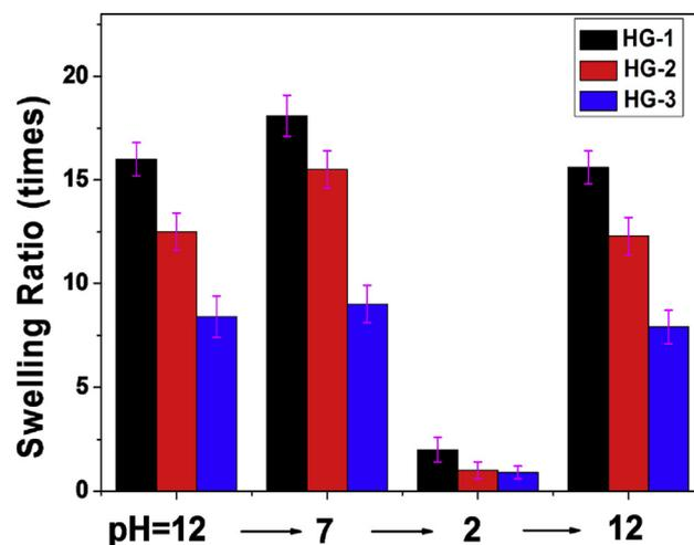
Fig. 3. Swelling ratio of hydrogels in water as a function of pH.
