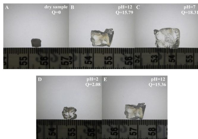
Fig. 4. Photographs of HG-1 with cyclic changing pH from 12 to 2 and back to 12.
