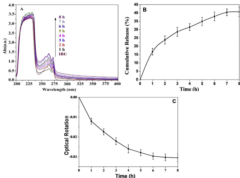
**Fig. 7.** (A) The UV–vis spectra of outer solution of ibuprofen released as a function of time; the curve of IBU represents the solution of 0.01 g IBU in 20 ml PBS. (B) Time–release profiles of ibuprofen of racemic IBU-loaded HG-1 in 20 ml PBS (pH, 7.4) determined according to UV–vis absorption. (C) Time–optical rotation of racemic IBU by HG-1 in 20 ml PBS (pH, 7.4).
