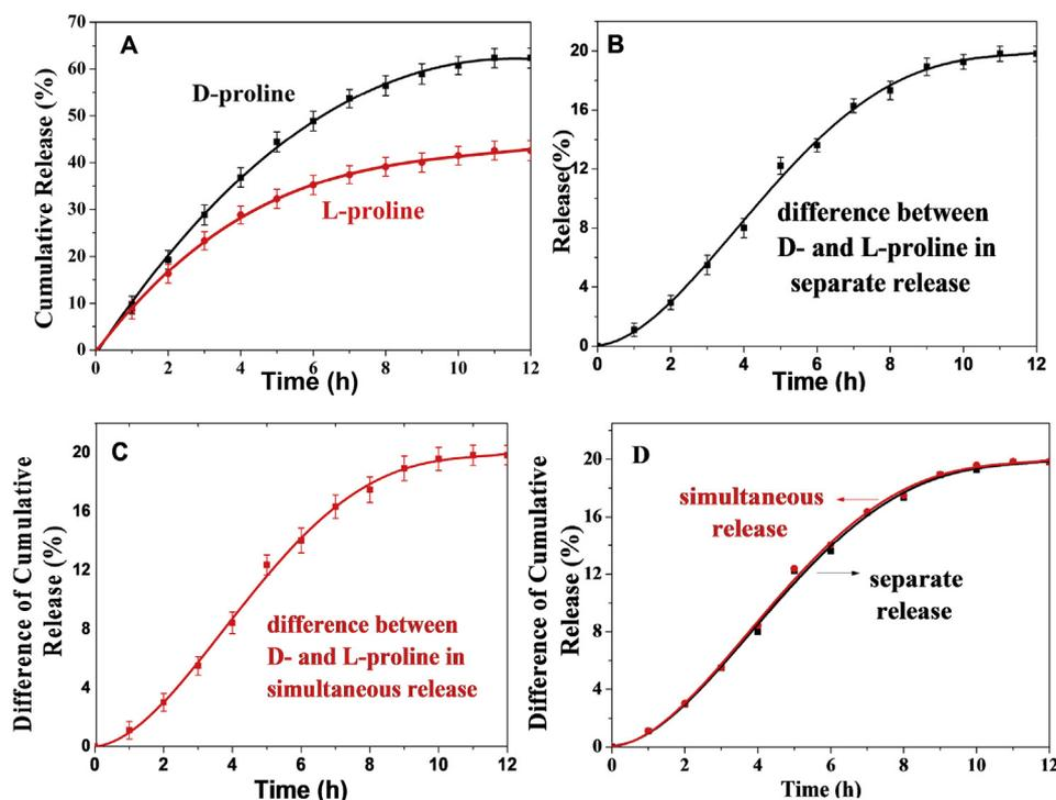
Fig. 6. Time-release profiles of L- and D-proline released by HG-1 in deionized water: L- and D-proline separately released (A) and the corresponding difference between L- and D-proline released (B); the difference between L- and D-proline when simultaneously released (C); a comparison of the difference between L- and D-proline released in the two cases (D), simultaneous release vs. separate release.
