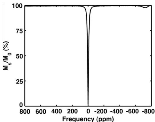
Figure 2. CEST spectrum of **4a** (23.4 mM in water containing 20% MeCN, room temperature, saturation power  $B_1$  30  $\mu\text{T}$ , presaturation time TS 3.9 s).
