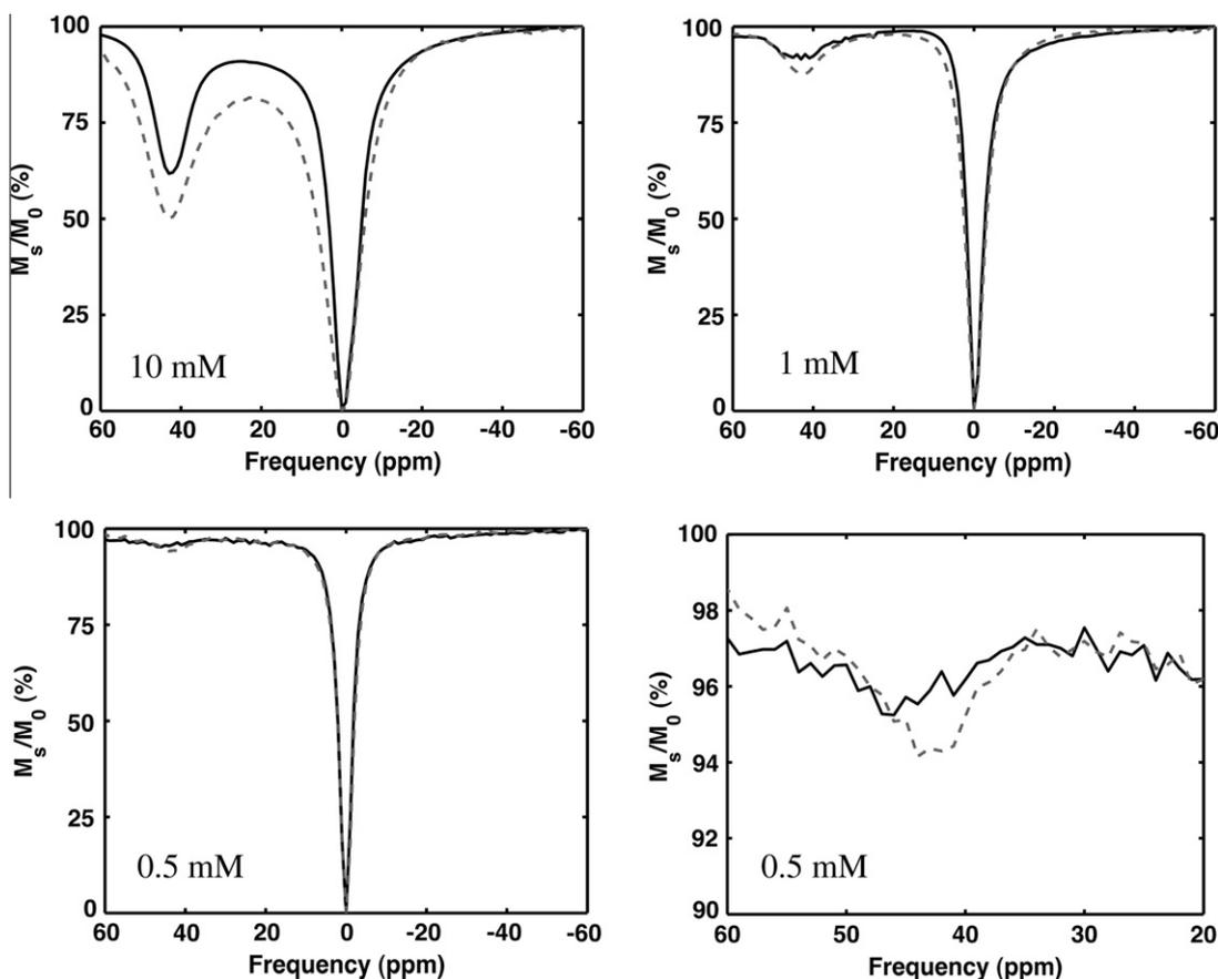
**Figure 4.** Comparison of the monomeric (**2b**) and dimeric europium-containing compounds (**4b**). CEST spectra (at 37 °C) of CAs **2b** (solid line) and **4b** (dashed line) at 10 mM (top left); 1 mM (bottom left) and 0.5 mM (top right). Expanded CEST spectrum at 0.5 mM (bottom right).
