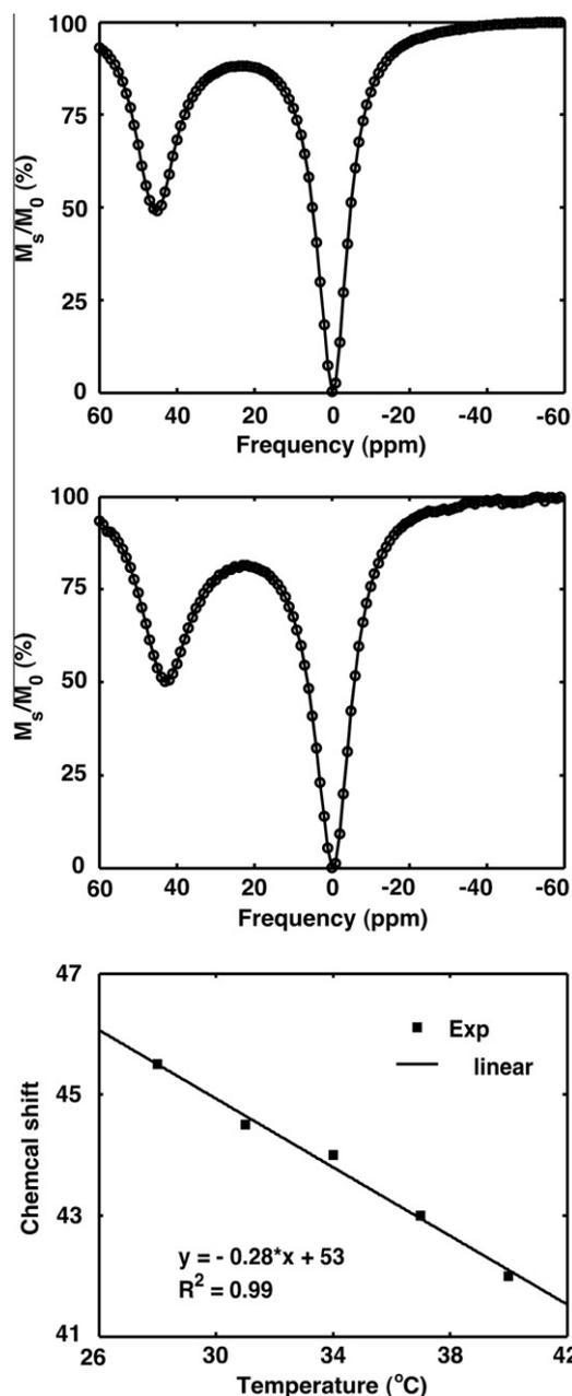
Figure 3. CEST spectra of the bimetallic PARACEST MRI CA **4b** at two temperatures (10 mM) at  $28^\circ\text{C}$  (top) and  $37^\circ\text{C}$  (middle) and the dependence of the bound water chemical shift on temperature (bottom).
