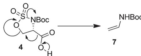
Scheme 3 Plausible route towards decomposition of sulfamidate **4**.
