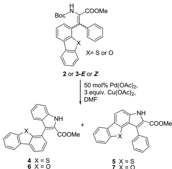
Scheme 2. Synthesis of heteroaryl and heteroannulated indoles **4–7** from the pure stereoisomers **2-E**, **2-Z**, **3-E**, and **3-Z**.
