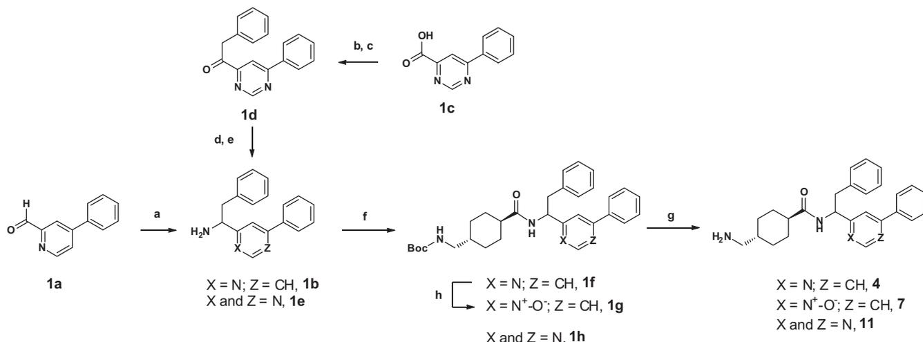
**Scheme 1.** Reagents and conditions: (a) LiHMDS, THF, 0 °C, then BnMgCl, 47%; (b) thionyl chloride, cat. DMF, DCE, reflux; (c) Pd(Ph<sub>3</sub>P)<sub>4</sub>, BnZnCl, THF, –30 °C to 0 °C, 43% over two steps; (d) hydroxylamine hydrochloride, MeOH; (e) Zn, TFA, 0 °C, 63% over two steps; (f) N-Boc-tranexamic acid, EDC, HOBt, Hunig's base, DMF, 0 °C to rt; (g) 30% TFA (v/v), CH<sub>2</sub>Cl<sub>2</sub>, rt, 45–67% over two steps. (h) mCPBA, CHCl<sub>3</sub>, rt.
