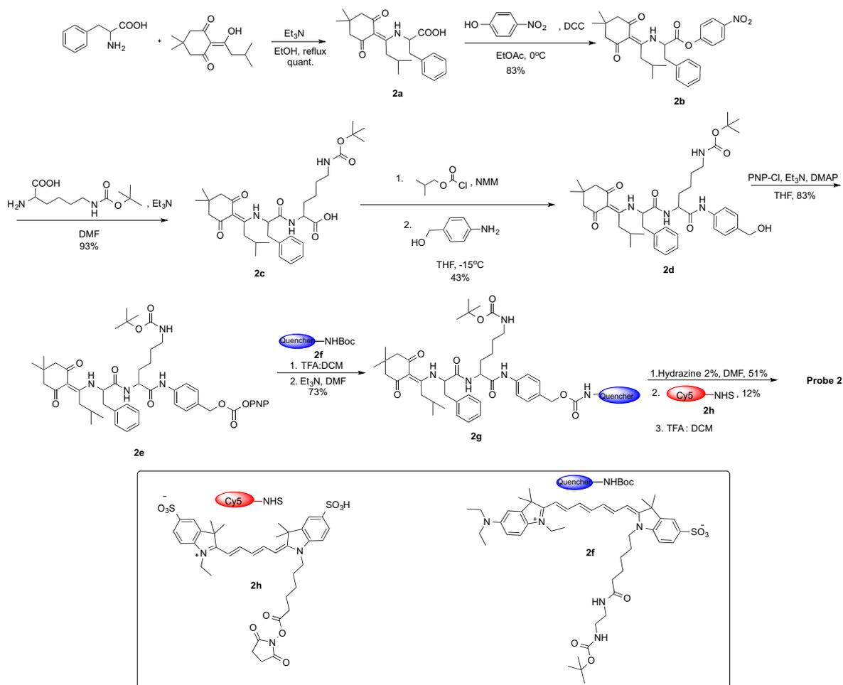
Figure 6. Chemical synthesis of probe **2**.
