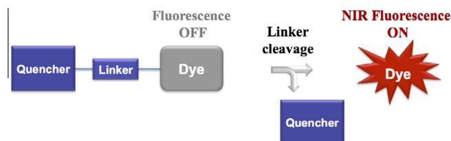
Figure 2. Illustration of the general design and mode of action of a FRET-based turn-ON probe.
