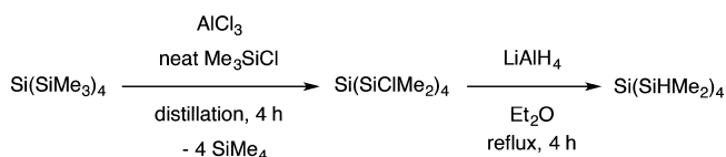
Scheme 1. Synthesis of Si(SiHMe 2 ) 4
