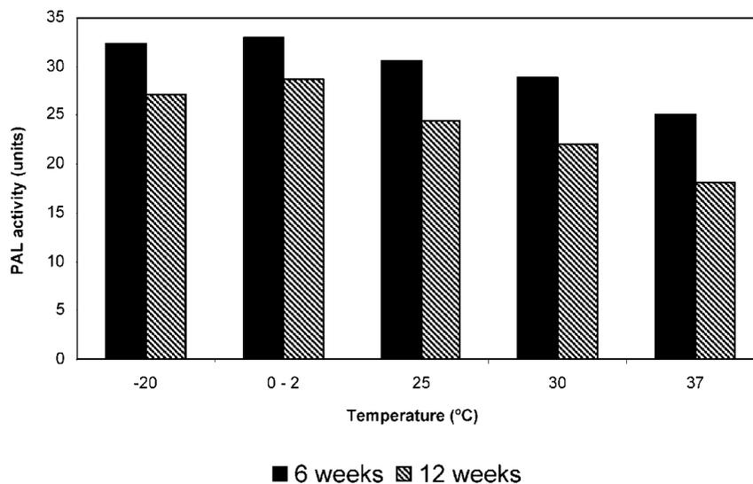
**Figure 2.** Effect of temperature on the storage stability of *R. glutinis* PAL. 0.01%  $Mn^{2+}$  was added to the storage buffer medium prior to adjustment of the pH to 8.8. Original PAL activity of *R. glutinis* cells was 34.0 units. PAL activity is reported in terms of units (nanomoles of L-Phe transformed per minute per milligram of dry cells).
