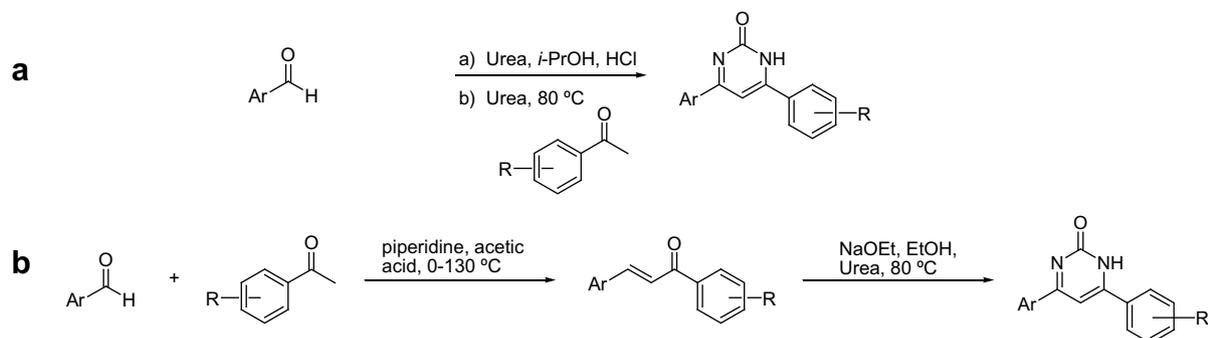
**Scheme 1.** Synthetic methods for pyrimidin-2(1H)-one series.
