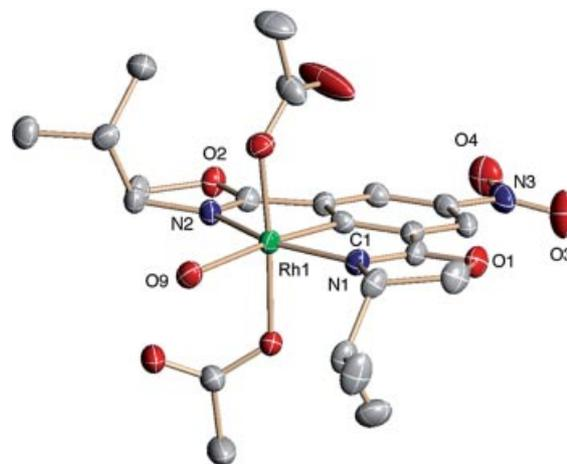
Figure 1. Molecular structure of complex **5a**. Selected bond lengths [Å] and angles [°]:  $\text{Rh1}-\text{C1}$  1.914(3),  $\text{Rh1}-\text{N1}$  2.055(3),  $\text{Rh1}-\text{N2}$  2.057(3),  $\text{Rh1}-\text{O9}$  2.195(2);  $\text{C1}-\text{Rh1}-\text{O9}$  174.38(12),  $\text{N1}-\text{Rh1}-\text{N2}$  159.00(10),  $\text{C1}-\text{Rh1}-\text{N1}$  79.72(12),  $\text{C1}-\text{Rh1}-\text{N2}$  79.29(12).
