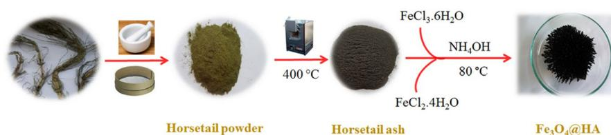
**Scheme 2** General route towards the synthesis of  $\text{Fe}_3\text{O}_4\text{@HA}$
