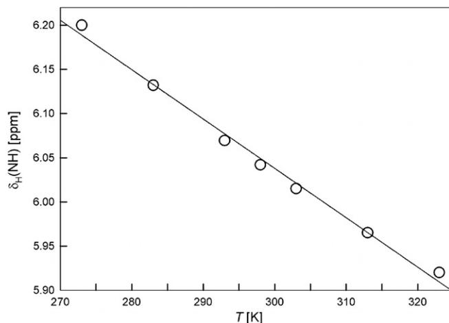
**Fig. 1.** Temperature dependence of amide proton chemical shift for urea (Sp)-2a. The spectra were recorded on a 0.01 M CDCl<sub>3</sub> solution and are referenced to tetramethylsilane. Solid line shows least-square linear fit of the data.
