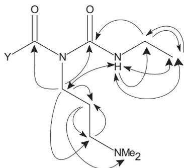
**Scheme 3.** Selected  $^{13}\text{C}$  gHMBC ( $\text{H} \rightarrow \text{C}$ ) and NOESY ( $\text{H} \leftrightarrow \text{H}$ ) correlations observed in the NMR spectra of  $(S_p)$ -**2b** (Y stands for the  $(S_p)$ -2-(diphenylphosphino)ferrocenyl group).
