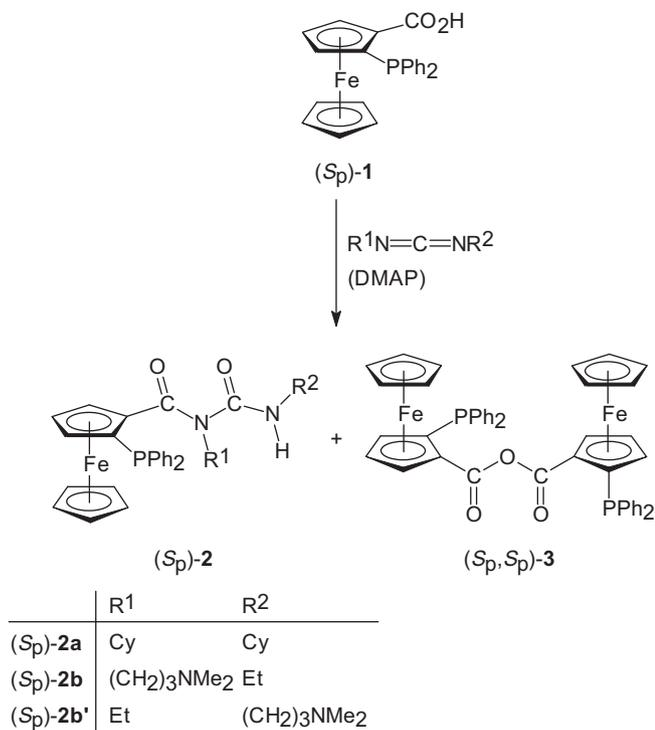
**Scheme 1.** The reaction of (Sp)-1 with diimides (DCC: R<sup>1</sup>/R<sup>2</sup> = Cy/Cy, EDC: R<sup>1</sup>/R<sup>2</sup> = Et/(CH<sub>2</sub>)<sub>3</sub>NMe<sub>2</sub>; Cy = cyclohexyl).
