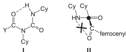
**Scheme 2.** A hypothetical planar, hydrogen-bonded conformation (I) and the conformation typically encountered in the crystal structures of compounds featuring C(ferrocenyl)C(O)N<sup>A</sup>CyC<sup>B</sup>(O)NHCy moiety (Cy = cyclohexyl) (II). For II, a projection along the N<sup>A</sup>...C<sup>B</sup> line is shown.
