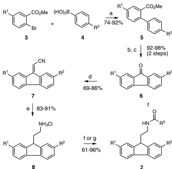
**Scheme 1.** Reaction conditions: (a) Pd<sub>2</sub>dba<sub>3</sub>, 2M Na<sub>2</sub>CO<sub>3</sub>, DME, 85°C, 16h; (b) 1N NaOH, EtOH, 78°C; (c) SOCl<sub>2</sub>, 79°C; (d) NCCH<sub>2</sub>PO(OEt)<sub>2</sub>, NaH, THF; (e) H<sub>2</sub>, PtO<sub>2</sub>, CHCl<sub>3</sub>, EtOH; (f) RCOCl or (RCO)<sub>2</sub>O, cat. DMAP, TEA, CH<sub>2</sub>Cl<sub>2</sub>; (g) RNCO, CH<sub>2</sub>Cl<sub>2</sub>.
