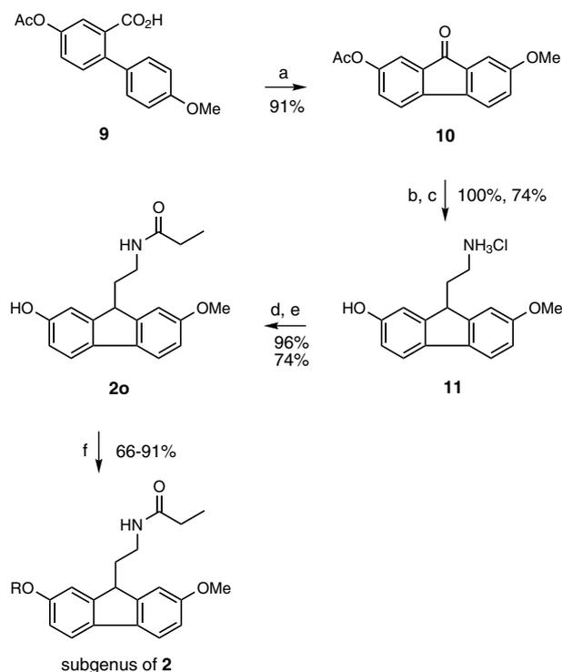
**Scheme 2.** Reaction conditions: (a) SOCl<sub>2</sub>, AlCl<sub>3</sub>; (b) NCCH<sub>2</sub>PO(OEt)<sub>2</sub>, NaH, DMF; (c) H<sub>2</sub>, Pd(C), CHCl<sub>3</sub>, EtOH; (d) RCOCl, TEA, cat. DMAP, CH<sub>2</sub>Cl<sub>2</sub>; (e) 1N NaOH, MeOH; (f) RI or RBr, K<sub>2</sub>CO<sub>3</sub>, MeCN.
