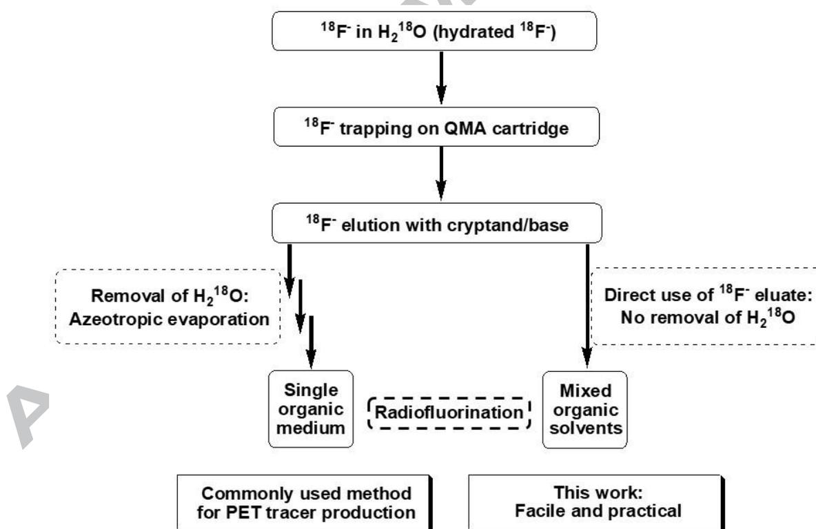
**Figure 1.** Radiofluorination with [ $^{18}\text{F}$ ]fluoride ions in a mixed organic solvent.
