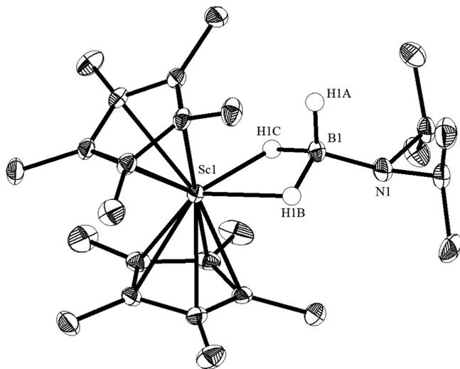
**Figure 2.** Molecular structure of complex **7**. Hydrogen atoms (except BH) are omitted for clarity, and ellipsoids are drawn at the 30% probability level. Selected bond lengths (Å) and angles (deg): Sc1–H1B, 2.02(2); Sc1–H1C, 1.95(2); B1–H1A, 1.18(2); B1–H1B, 1.22(3); B1–H1C, 1.22(3); B1–N1, 1.491(3); H1B–Sc1–H1C, 53.4(11); H1B–B1–H1C, 94.4(17).
