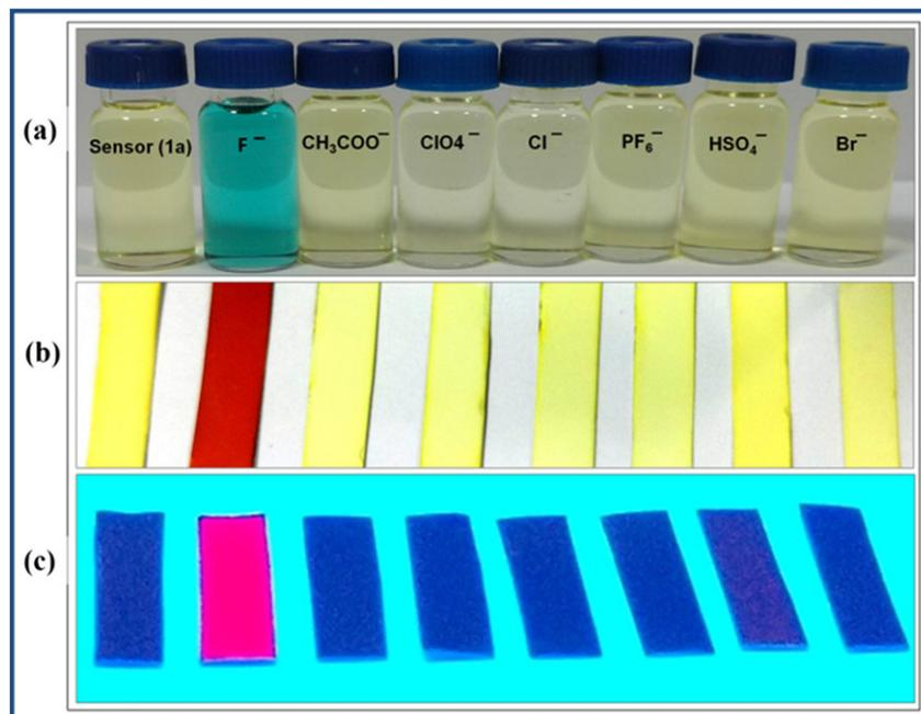
**FIGURE 9** Demonstration for F<sup>-</sup> ions sensing (a) Solutions colours of (1) in the presence of various anions (b) Strips colour under the white light (c) Strips colour under the UV light (long wavelength)
