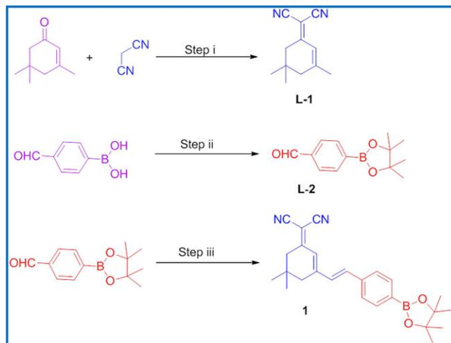
**SCHEME 1** Synthesis of Boron based chemosensor (**1**). Reagents and reaction conditions used: Step (i): Piperidine, Dry Ethanol, 60 °C, 8 hours. Step (ii): L-1, Pinacol, Diethyl ether, 25 °C, 24 hrs. Step (iii): Knoevenagel Condensation of L-1 and L-2, Dry Ethanol, 40 °C, 8 hrs
