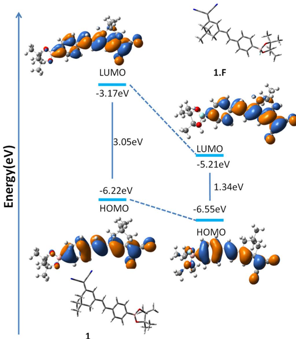
**FIGURE 6** DFT energy levels diagram of (**1**) and (**1.F**)<sup>-</sup>
