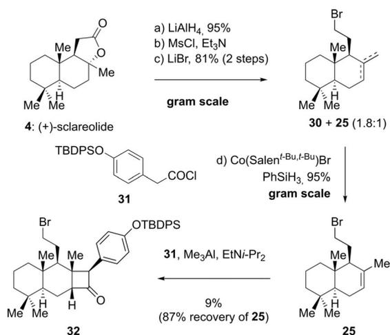
**Scheme 5.** Construction of  $\alpha$ -arylcyclobutanone **32** through ketene-based [2+2] cycloaddition.
