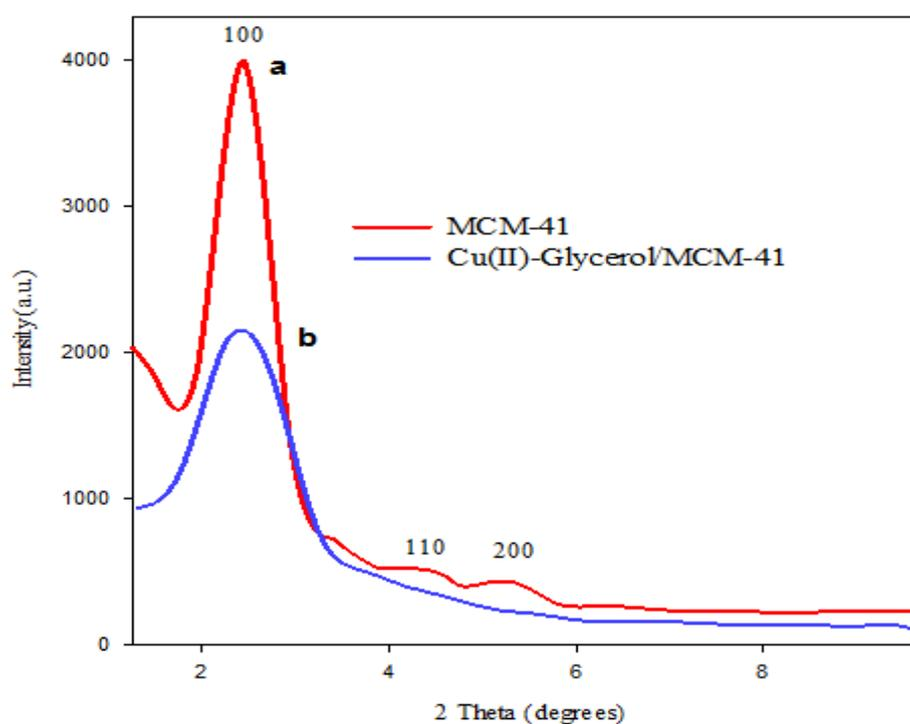
**Figure 3.** Low-angle powder XRD pattern of (a) MCM-41 and (b) Cu(II)-Glycerol/MCM-41
