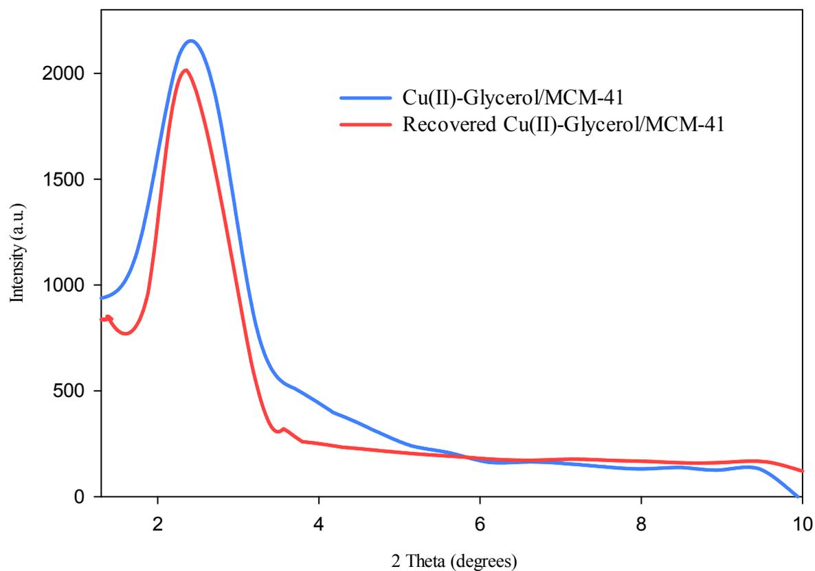
**Figure 8.** XRD pattern of recovered Cu (II)-Glycerol/MCM-41 nanocatalyst
