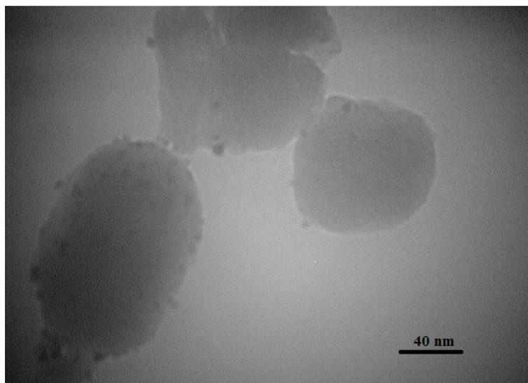
**Figure 9.** TEM image of recovered Cu (II)-Glycerol-MCM-41 nanocatalyst
