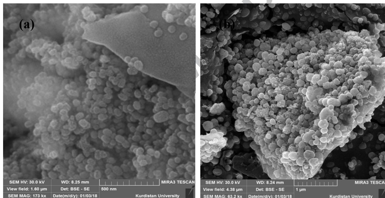
**Figure 1.** SEM of the synthesized MCM-41 (a) and Cu(II)-Glycerol/MCM-41 (b)
