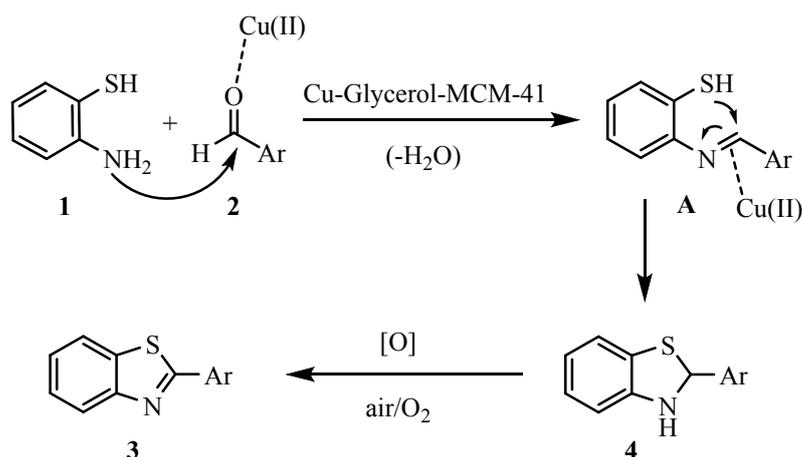
**Scheme 2.** Proposed mechanism for the synthesis of benzothiazoles in the presence of Cu(II)-Glycerol-MCM-41
