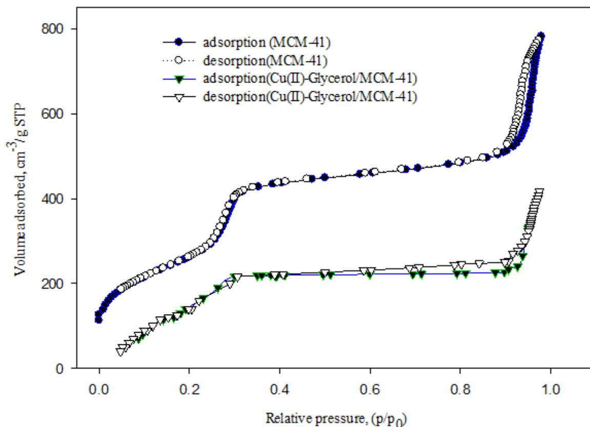
**Figure 5.** N<sub>2</sub> adsorption–desorption isotherms for, (a) MCM-41 and (b) Cu(II)-Glycerol/MCM-41
