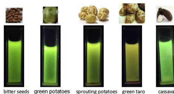
Fig. 12. Solution color changes under 365 nm UV lamp of sensor 3TI to monitor cyanide in food samples. (For interpretation of the references to color in this figure legend, the reader is referred to the Web version of this article.)
