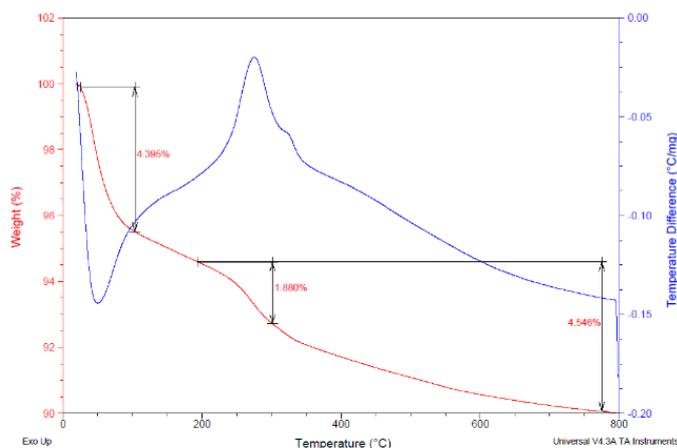
Figure 6. Thermal analysis of Co/SiO<sub>2</sub> catalyst after reaction.
