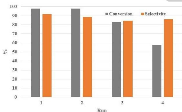
**Figure 4.** Evolution of the xylose conversion and xylitol selectivity with reaction cycle number. Reaction conditions: 140°C, 5.0 MPa of hydrogen, 2 h of reaction, 5 wt.% of xylose, 10 mL of water, 5 wt.% of catalyst with respect to xylose mass.
