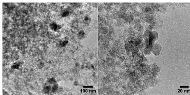
**Figure 2.** TEM images recorded for reduced Co/SiO<sub>2</sub> catalyst.
