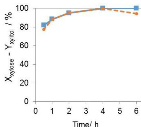
**Figure 3.** Hydrogenation of xylose to xylitol in the presence of Co/SiO<sub>2</sub> catalyst (full line: xylose conversion; dotted line: xylitol yield).
