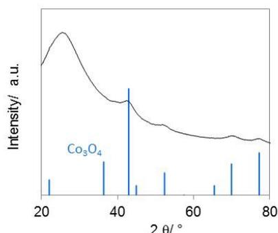
**Figure 1.** XRD analysis of Co/SiO<sub>2</sub> catalyst before (vertical bars, reference ICDD 42-1467).
