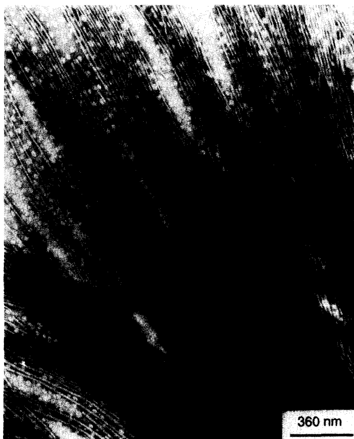
Fig. 3. Electron micrograph of compound 18b in the presence of urea after sonication (negative staining by phosphotungstic acid).
