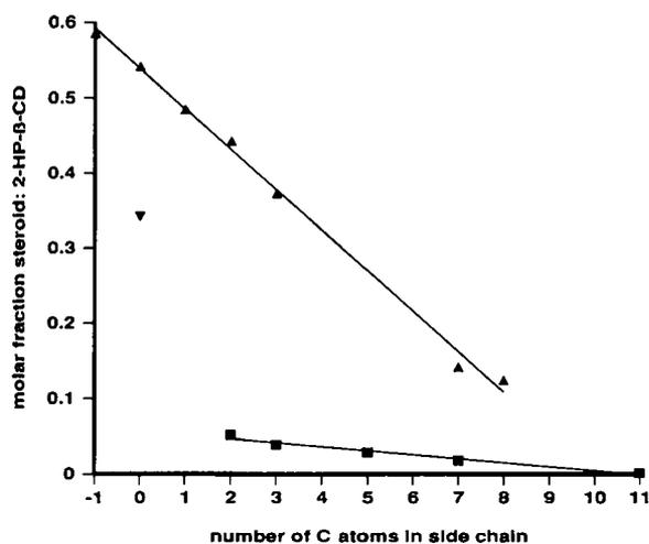
**Figure 4—Dependence of the solubilization of steroid hormone esters with 2-HP- $\beta$ -CD on the number of C atoms in the ester side chain for various testosterone esters ( $\blacktriangle$ ), estradiol esters ( $\blacksquare$ ), and estradiol ( $\blacktriangledown$ ).**
