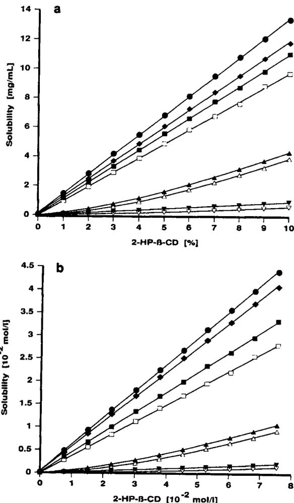
**Figure 1**—Phase solubility diagram of methyltestosterone (●), testosterone (◆), testosterone 17-acetate (◆), testosterone 17-propionate (□), testosterone 17-enanthate (▲), testosterone 17-cypionate (△), cyproterone acetate (▼), and testosterone 17-benzoate (▽) with 2-HP- $\beta$ -CD in pH 7.4 phosphate buffer at 25  $^\circ\text{C}$  (a) 2-HP- $\beta$ -CD expressed in percent; (b) 2-HP- $\beta$ -CD expressed in molar concentration.
