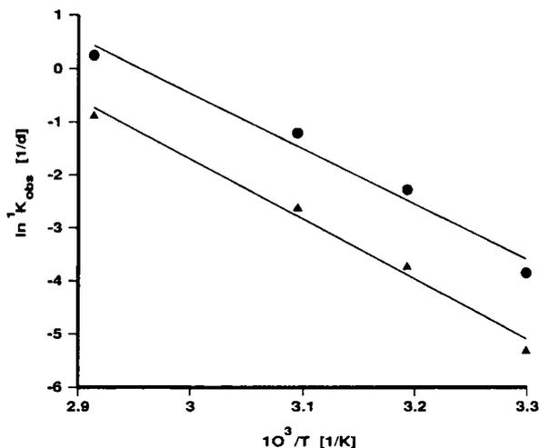
**Figure 7**—Arrhenius diagram for the decomposition of testosterone acetate at pH 9 in methanolic aqueous solution (●) and in 2% aqueous 2-HP-β-CD (▲) (d, days; T, temperature).
