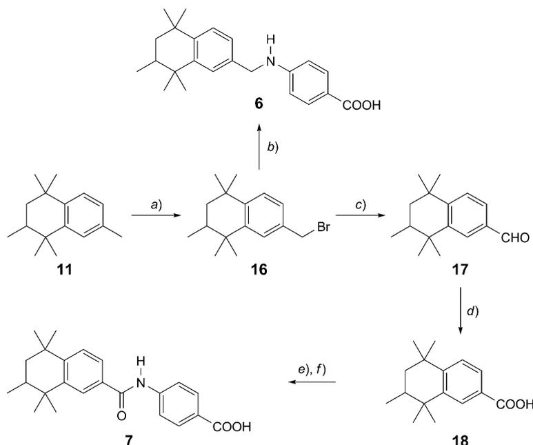
a) *N*-Bromosuccinimide (NBS),  $\text{CCl}_4$ , reflux. b) *p*-Aminobenzoic acid (PABA), acetone, anh.  $\text{K}_2\text{CO}_3$ , reflux. c) Hexamethylenetetramine 1,3,5,7-tetraazatricyclo[3.3.1.1<sup>3,7</sup>]decane; HMT,  $\text{CHCl}_3$ , reflux, 50% gl. AcOH and HCl. d)  $\text{KMnO}_4$ ,  $\text{H}_2\text{O}$ , 70–80°. e)  $\text{SOCl}_2$ , 45–50° f) PABA, pyridine.
