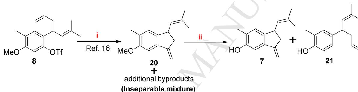
**Scheme 6:** Reagents and conditions: (i) Pd(PPh<sub>3</sub>)<sub>4</sub>, TEA, LiCl, DMF, 110 °C, 20 h; (ii) EtSH, NaH, DMF, 130-140 °C, 24 h, 56% (**7**) and 14% (**21**) over two steps.
