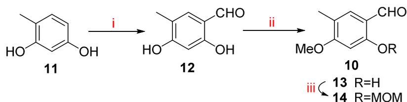
**Scheme 4:** Reagents and conditions: (i)  $\text{POCl}_3$ , DMF, MeCN, 0 °C to rt, 5 h, 93%; (ii) Dimethylsulphate,  $\text{K}_2\text{CO}_3$ , MeCN, rt, 12 h, 95%; (iii) MOMCl, NaH, THF, 0 °C, 30 min, 94%.
