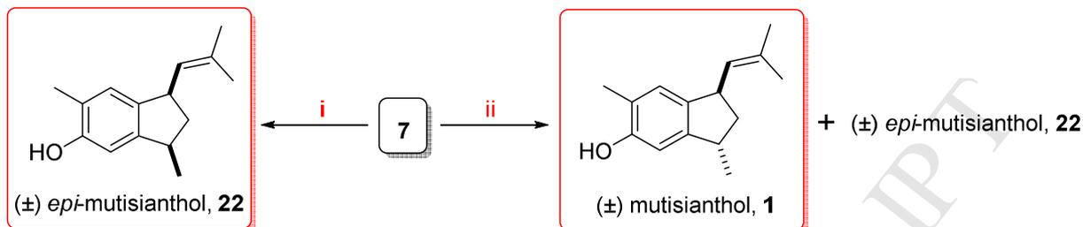
**Scheme 7:** Reagents and conditions: (i) H<sub>2</sub> (balloon), 10% Pd/C, MeOH, rt, 1 h, 84%; (ii) (a) MOMCl, DIPEA, DCM, 0 °C to rt, 12 h, 86%; (b) Li, liq. NH<sub>3</sub>, THF -78 °C, 12 h, then 6 N HCl, 40% (**1**) and 40% (**22**).
