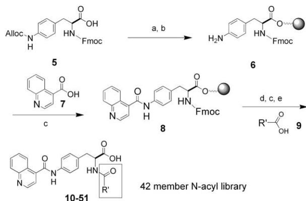
**Scheme 1.** (a) Wang resin, BOP, NMP; (b) Pd(Ph<sub>3</sub>P)<sub>2</sub>Cl<sub>2</sub>, *N*-Bu<sub>3</sub>SnH, HOAc, DCM, rt; (c) acid **7**, BOP, DIEA, NMP, rt; (d) 25% piperidine, NMP, rt; (e) 90% TFA, DCM, rt.
