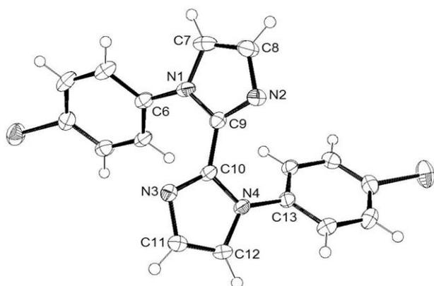
**Figure 1** ORTEP plot (50% probability ellipsoids) of the solid-state molecular structure of biimidazole **3b**. Selected bond lengths (Å): N1–C6 1.424(3), N1–C7 1.384(4), N1–C9 1.373(3), N2–C8 1.373(3), N2–C9 1.315(3), C9–C10 1.469(3), N3–C10 1.313(3), N3–C11 1.378(3), N4–C10 1.371(3), N4–C12 1.381(3), N4–C13 1.431(3), C7–C8 1.343(4), C11–C12 1.359(4)
