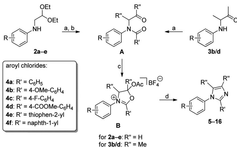
Scheme 4. Preparation of 1,2-diarylimidazoles. Reagents and conditions: (a) **4a–4f**, NEt<sub>3</sub>, dichloromethane (DCM), room temp., (b) *para*-toluenesulfonic acid (*p*-TsOH), acetone/H<sub>2</sub>O (9:1), reflux, (c) HBF<sub>4</sub> (aq.), acetic anhydride (Ac<sub>2</sub>O), room temp., (d) NH<sub>4</sub>OAc, HBF<sub>4</sub> (aq.), CH<sub>3</sub>CN, room temp. to reflux.
