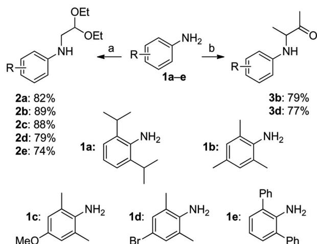
Scheme 3. Syntheses of alkylated anilines. Reagents and conditions: (a) *n*BuLi, bromoacetaldehyde diethyl acetal, tetrahydrofuran (THF), room temp., (b) 2-hydroxybutanone, cat. HCl, toluene, reflux.
