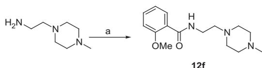
**Scheme 2.** Reagents and conditions: (a) 2-Methoxybenzoyl chloride, pyridine, 50 °C, 24 h, 72%.
