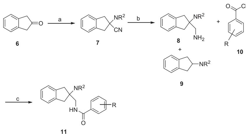
**Scheme 1.** Reagents and conditions: (a) TMSCN, ZnI<sub>2</sub>, Et<sub>2</sub>O, NHR<sub>2</sub>, MeOH, 80 °C, 8 h, 50–90%; (b) LAH, Et<sub>2</sub>O, THF, 2 h, reflux, 0–70% or LAH, H<sub>2</sub>SO<sub>4</sub>, Et<sub>2</sub>O, 5 h, reflux, 0–75%; (c) Pyridine, 50 °C, 24 h, 15–65%.
